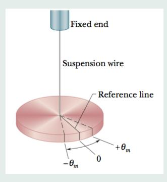
• **Resoring torque:** from twisting of the suspension wire
