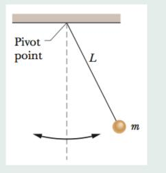
• Restoring force = tangential component of gravitational force
