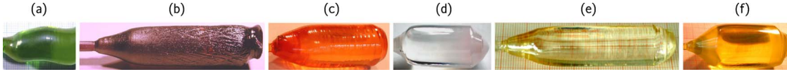
FIG. 1. (Color online) Photographs of single-crystal rare-earth scandates grown along the [110] direction by the Czochralski method. (a) \text{PrScO}_3 with a diameter of 12 mm, (b) \text{NdScO}_3 with a diameter of 16 mm, (c) \text{SmScO}_3 with a diameter of 18 mm, (d) \text{GdScO}_3 with a diameter of 32 mm, (e) \text{TbScO}_3 with a diameter of 18 mm, and (f) \text{DyScO}_3 with a diameter of 32 mm.
