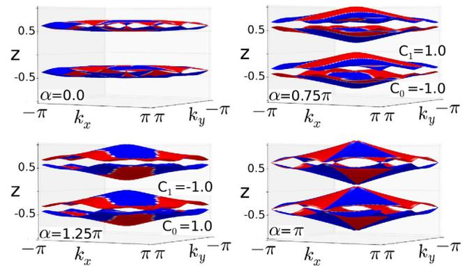
FIG. 1 (color online). The two WCC sheets of the half filled FKM model, and one set of periodic images, at four stages  $\alpha = (0, 3\pi/4, \pi, 5\pi/4)$  along the parametric cycle (clockwise from upper left). Blue and red colors show positive and negative values of Berry curvature  $\Omega_z$  on the sheets, respectively. The Chern numbers associated with the individual WCC sheets are shown for those cases where sheets do not touch.
