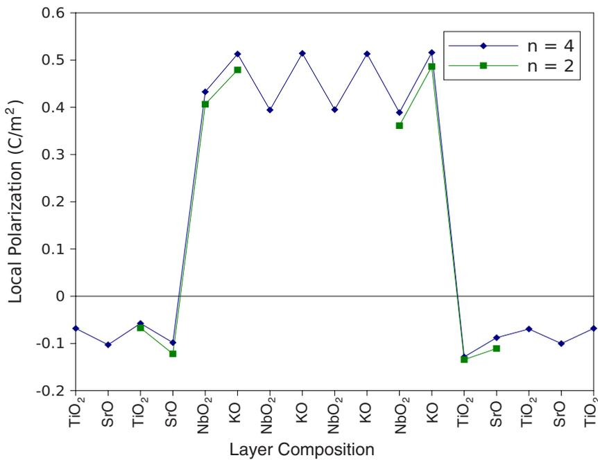
FIG. 4. (Color online) Layer-by-layer local polarization profile of a supercell with  $n=4$  (four  $\text{SrTiO}_3$  units and four  $\text{KNbO}_3$  units), with corresponding results for  $n=2$  also indicated near each of the interfaces.
