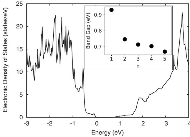
FIG. 3. Calculated electronic density of states for a supercell with  $n=2$  (two SrTiO<sub>3</sub> layers and two KNbO<sub>3</sub> layers). Inset shows the gradual reduction in band gap for  $n$ SrTiO<sub>3</sub>/ $n$ KNbO<sub>3</sub> supercells as  $n$  increases.
