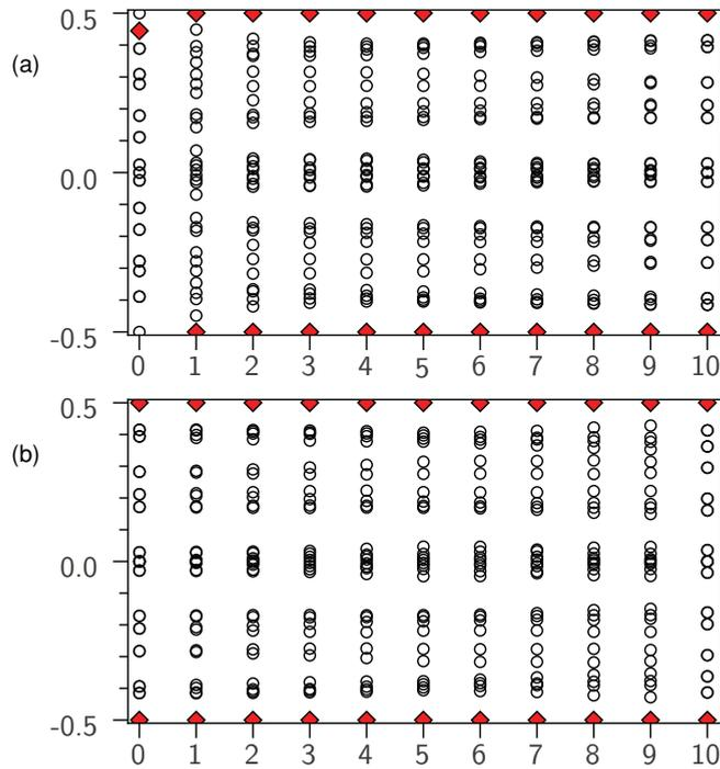
FIG. 4. (Color online) Evolution of  $\text{Bi}_2\text{Se}_3$  WCCs  $\bar{x}_n$  (circles) in the  $r_3$  direction vs  $k_2$  at (a)  $k_1 = 0$ ; (b)  $k_1 = \pi$ . Red rhombus marks midpoint of largest gap.  $k_2$  is sampled in 10 equal increments from 0 to  $\pi$ .
