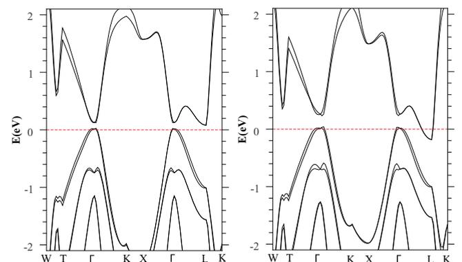
FIG. 6. (Color online) Band structure along high-symmetry lines of the undistorted fcc structure for HgTe under tensile strain in the [111] direction. (a)  $+2\%$  strain. (b)  $+5\%$  strain.
