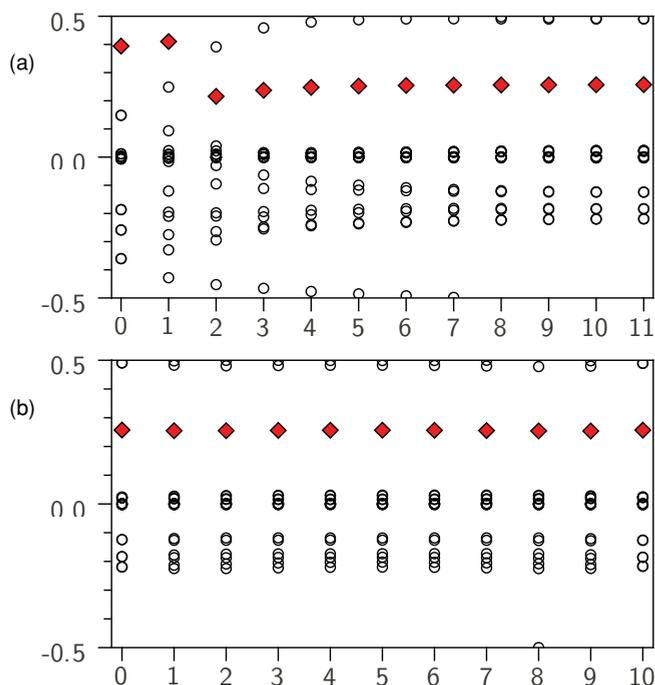
FIG. 7. (Color online) Evolution of WCCs for HgTe under +2% strain in the [111] direction. WCCs  $\bar{x}_n$  (circles) in the  $r_3$  direction are plotted vs  $k_2$  at (a)  $k_1 = 0$ ; (b)  $k_1 = \pi$ . Red rhombus marks midpoint of largest gap.  $k_2$  is sampled in 10 equal increments from 0 to  $\pi$ , except that an extra point is inserted midway in the first segment in panel (a) (see the text).
