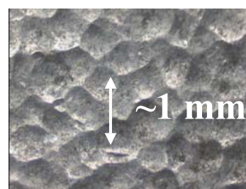
Figure 2b. A photomicrograph of the peened surface of the 3.85 mm thick specimen.
