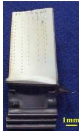
Figure II-4d. A photograph of a turbine blade. Note the complex hole cooling patterning emphasizing the need for engineering intensive design to maintain strength in an ultrahigh temperature environment. Proceedings of the 2007 Residual Stress Summit.)
