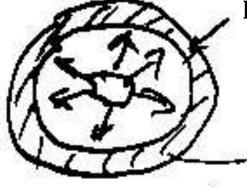
high Z material resists expansion by virtue of the inertia of its mass (tamper)
