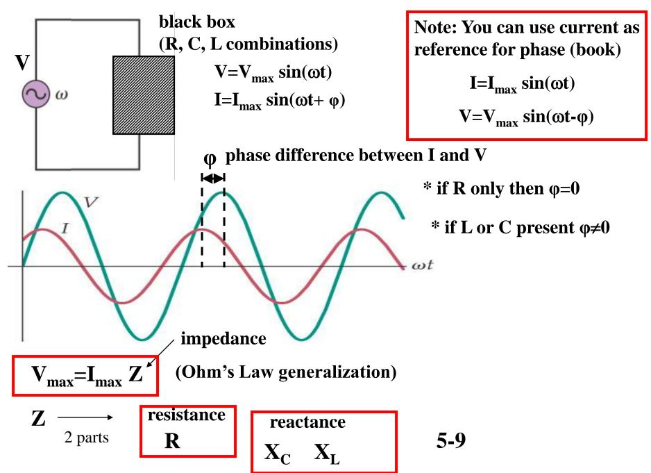
$$I = I_{0} \sin(\omega t) \Rightarrow V = V_{0} \sin(\omega t \pm \phi)$$
