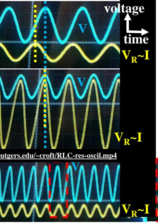
$\omega << \omega_0$ I small  $Z \sim \sqrt{\left[-\frac{1}{\omega C}\right]^2}$ phase C -like
