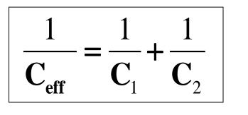
$\frac{1}{C_{eff}} = \frac{1}{C_1} + \frac{1}{C_2} + \frac{1}{C_3} + \dots$
