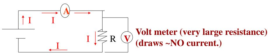
DC (direct current ) multi-meters measures volts & amps.
