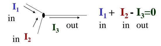
The sum of the currents into any junction must equal zero.
