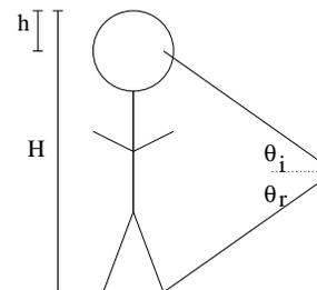
Since the angle of incidence equals the angle of reflection, the person's feet will be visible when the bottom of the mirror is *half* the distance between her eyes and the floor. (See the extraordinarily well-rendered figure above.) If her height is  $H$  meters and her eyes are  $h$  meters from the top of her head, this means that
