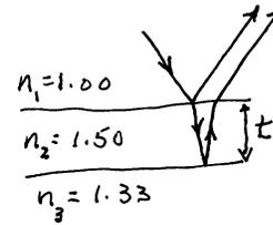
Reflected wave has half-cycle phase shift at top interface, and no phase shift at bottom interface. For constructive interference,
