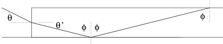
The figure above shows a little more detail than the figure attached to the problem. Using trigonometry, we know that  $\phi$  is related to the angle of refraction as the light enters the film  $\theta' = 90^\circ - \phi$ , and that if total internal reflection occurs at both surfaces,  $\phi$  must be greater than or equal to the critical angles at both surfaces. The film-air critical angle is
