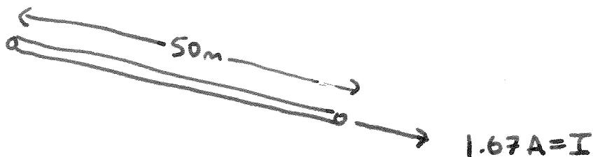
$$E = \rho \frac{J}{l} = \underbrace{(1.72 \times 10^{-8} \Omega m)}_{\rho} \times \underbrace{\left( \frac{1.67 A}{8.2 \times 10^{-7} m^2} \right)}_{J/l}$$
