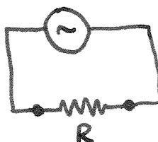
$$\begin{aligned} V_R &= iR = (IR) \cos \omega t \\ &= V_R \cos \omega t \end{aligned}$$
