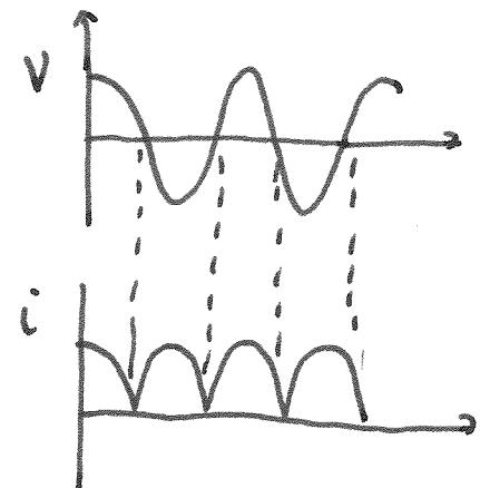
Current only flows one way through the galvanometer.
