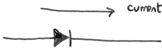
A diode only transmits a current in the direction of the arrow.
