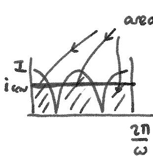
$$= 4 \int_0^{\pi/2\omega} I \cos \omega t dt = \frac{\frac{4I}{\omega}}{\frac{2\pi}{\omega}}$$
