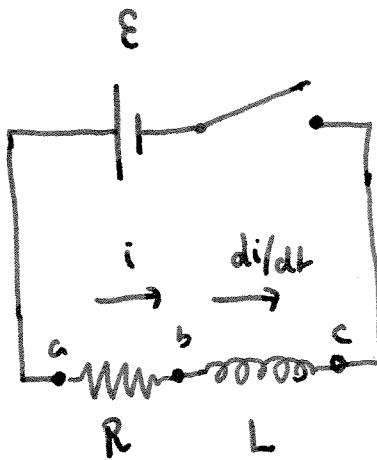
$$\left. \begin{array}{l} V_{ab} = iR \\ V_{bc} = L \frac{di}{dt} \end{array} \right\} \text{At } t=0 \quad i=0 \text{ - requires time to build up}$$
