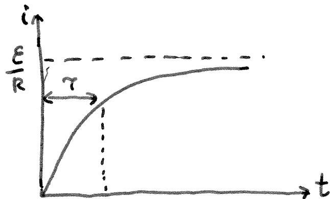
$$\text{e.g. } R = 1\Omega, L = 1\text{mH} \quad \tau = \frac{1\text{mH}}{1\Omega} = \underline{\underline{1\text{ms}}}$$
