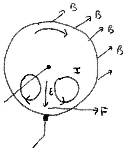
Notice in second example direction of  $\vec{F} = I \vec{L} \times \vec{B}$  provides a breaking torque.
