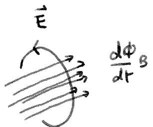
The minus sign tells us that the sense of rotation around the increasing flux is left-handed.
