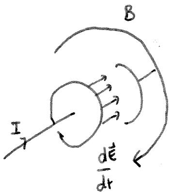
$$\oint \vec{B} \cdot d\vec{l} = \mu_0 \left( I + \underbrace{\epsilon_0 \frac{d\Phi_E}{dt}}_{\text{displacement}} \right)_{\text{encl}}$$
