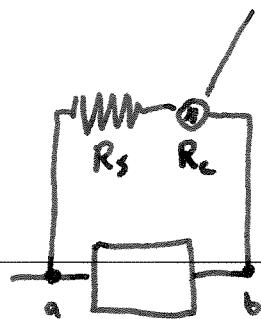
$$\begin{array}{c} \text{full swing voltage} \\ \downarrow \\ V_{ab} = (R_s + R_g) I_{sf} \\ \downarrow \\ \text{full swing current.} \end{array}$$
