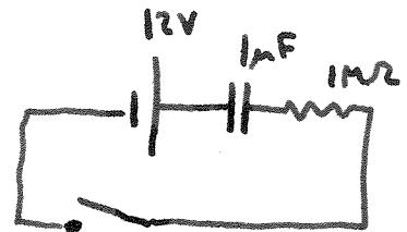
e.g Resistor with  $R = 1\text{M}\Omega$  in series +  $1\mu\text{F}$
