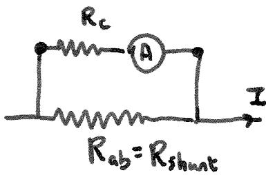
$$\begin{aligned} V &= I_{fs} R_c \\ &= (I - I_{fs}) R_{ab} \\ \Rightarrow I_{fs} (R_c + R_{ab}) &= I R_{sh} \end{aligned}$$
