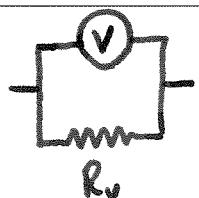
Voltmeter + finite resistance
