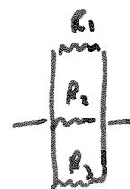
$$I = I_1 + I_2 + I_3 = \frac{V_{ab}}{R_1} + \frac{1}{R_2} + \frac{1}{R_3}$$
