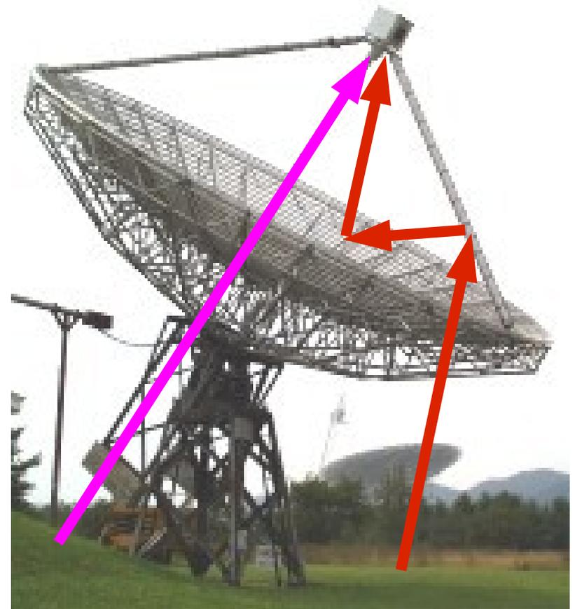
“Spillover” occurs when emission from “behind” telescope enters main beam due to **reflection off supports** and/or the fact that the feed “sees” **beyond the edge of the dish.**
