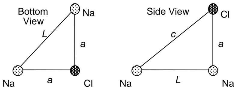
The length,  $L$ , of the diagonal of the bottom face of the cube can be found using the Pythagorean theorem to be
