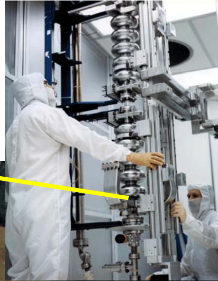
Superconducting radiofrequency (SRF) cavities undergo vertical testing.
