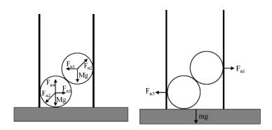
For the top ball,  $Mg = \frac{F_{n_2}}{\sqrt{2}}$  and  $F_{n_1} = \frac{F_{n_2}}{\sqrt{2}}$ . Thus,  $F_{n_1} = Mg$  and  $F_{n_2} = \frac{Mg}{\sqrt{2}}$ .
