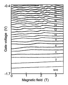
FIG. 2. Plot of the gate voltage positions of the current oscillations vs magnetic field for a dot with  $D = 0.5 \ \mu m$ .
