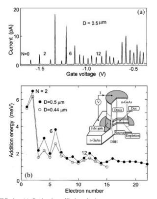
FIG. 1. (a) Coulomb oscillations in the current vs gate votage at B = 0 T observed for a  $D = 0.5 \ \mu \text{m}$  dot. (b) Addition energy vs electron number for two different dots with D = 0.5 and 0.44  $\mu \text{m}$ . The inset shows a schematic diagram of the device. The dot is located between the two heterostructure barriers.
