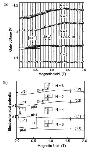
FIG. 4. (a) Evolution of the third, fourth, fifth, and sixth current peaks with *B* field from 0 to 2 T observed for the  $D = 0.5 \ \mu \text{m}$  dot shown in a manner described for Fig. 3(b). (b) Calculated electrochemical potential vs magnetic field for the model described in the text and parameters U = 3 meV,  $\Delta = 0.7 \text{ meV}$ , and  $\hbar \omega_0 = 3 \text{ meV}$ .
