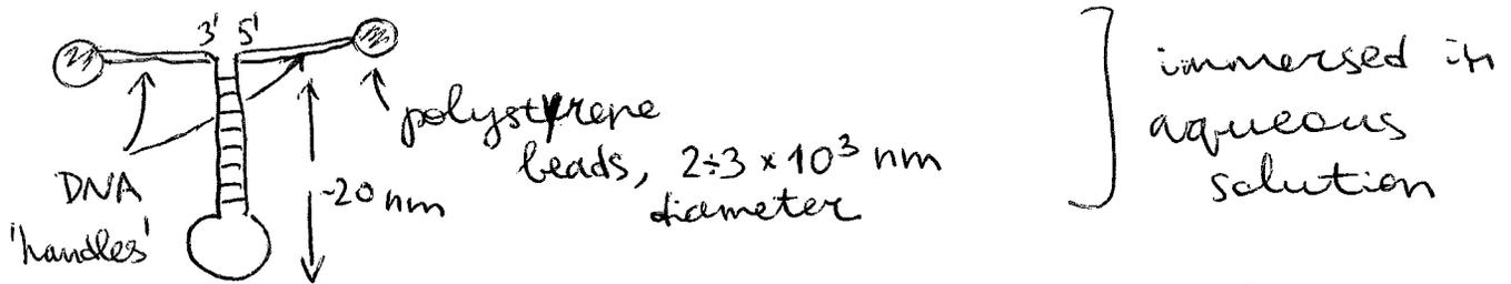
One lead anchored on a glass micropipette, the other one confined by an optical trap. You control the displacement of the RNA molecule ( $\Delta$ ) and can measure forces acting on the lead.
