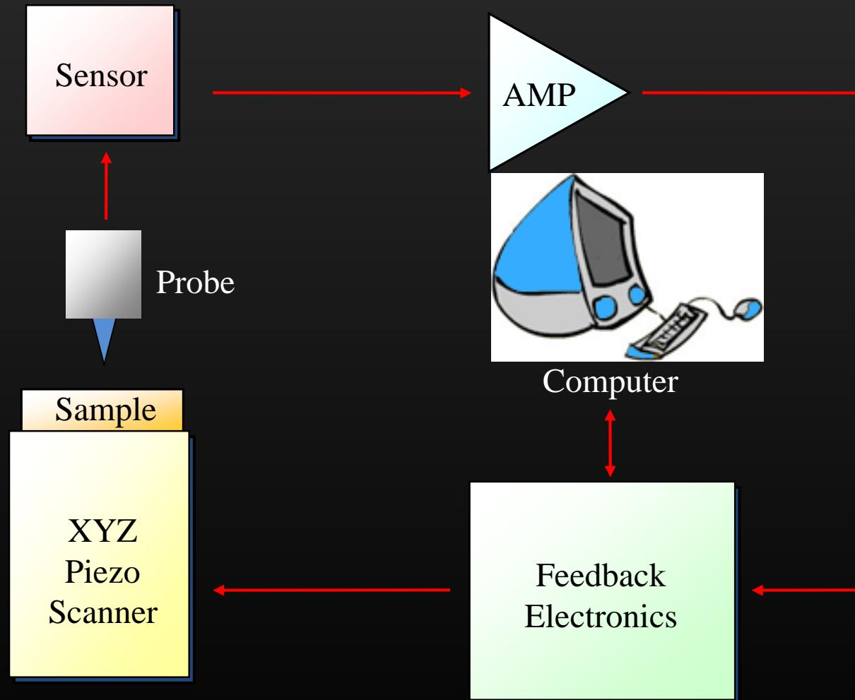
Probe signal: tunneling, force, optical, thermal, capacitance ...
