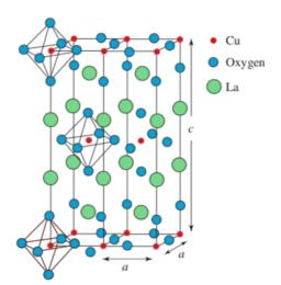
Fig. 1 Crystal structure of La<sub>2</sub>CuO<sub>4</sub>, showing bodycentered tetragonal conventional cell
