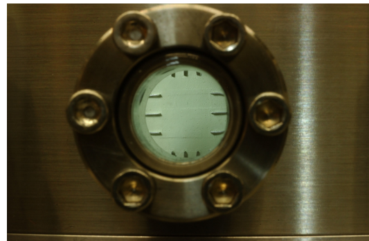
Figure 8. Image of the phosphor plate with edges populated with fiducial markings.
