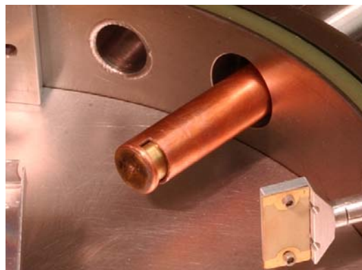
Fig. 8 Displaying older Faraday collector showing thick RF shielded tip (left) and the fluorescent screen at the bottom right). Ion rotation is obviously CCW (counter clockwise).
