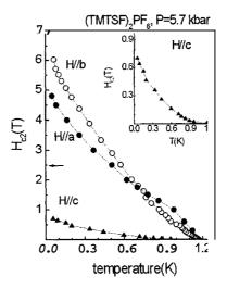
Figure 1. Resistively determined critical field along the principle axes for (TMTSF)2PF6. Insert is expansion of c axis data. All curves are well above the calculated Ginzburg-Landau values. Horizontal arrow indicates the Pauli limiting field for singlet superconductivity.
