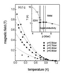
Figure 2. C axis critical field for several pressures near the SDW-superconducting phase boundary. Insert – measured phase diagram with vertical lines indicating samples shown in main plot.
