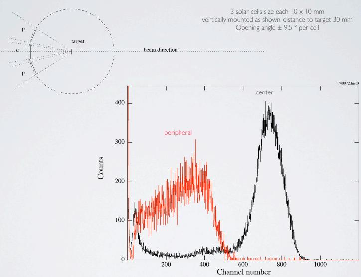
Spectra taken with the same preamplifier (same gain) . Both peripheral cells were wired together. Center and peripheral give nearly the same slopes and the rates are for all cells more or less the same. Conclusion: it does not pay to separate the particle detector and have the added data handling.
