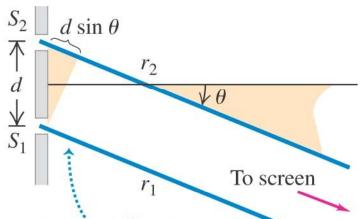
... so we can treat the rays as parallel, in which case the path-length difference is simply  $r_2 - r_1 = d \sin \theta$ .
