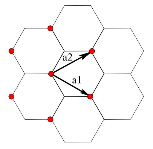
Figure 1: The lattice structure of graphene is a honeycomb lattice.
