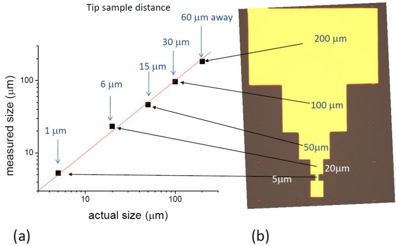
FIG. 3. (Color on line) Sample widths measured by the capacitance method illustrated in Fig.2. (a) Measured size versus actual size. Tip sample distances adjusted for sharp edge resolution corresponding to aspect ratios of 0.3 or less. Red line is a guide to the eye through the values of the measured widths. (b) Optical image of sample.
