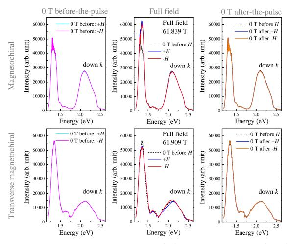
FIG. S2: Power spectra of  $Ni_3 TeO_6$  in both the magnetochiral (top) and transverse magnetochiral (bottom) orientations. The first plot in each series is the 0 T power spectra before the magnet pulse. The second plot is the full field power spectra for the respective orientations. The final plot is the 0 T power spectra after the magnet pulse compared to 0 T spectra before the magnet pulse. This eliminates hysteretic concerns.
