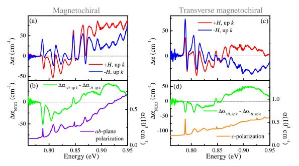
FIG. S7: (a, c) Close-up of  $\Delta \alpha$  in the magnetochiral and transverse magnetochiral orientations at 4.0 K. (b, d)  $\Delta \alpha_{NDD}$  in the different measurement orientations with the linear absorption spectrum plotted underneath for reference. Clearly, a number of the phonons display nonreciprocal effects.
