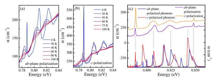
FIG. S6: (a, b) Close-up view of the fine structure on the optical absorption as a function of temperature in the ab-plane and c-direction. (c) Close-up view of the optical absorption in the vicinity of the fine structure. The phonon spectra [S17] are plotted underneath for comparison.
