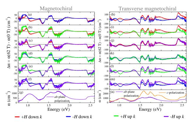
FIG. S3: Full field absorption difference  $(\Delta \alpha)$  spectra for each comparison are plotted, with the (+H, down k) in red, (-H, down k) in blue, (+H, up k) in green, and (-H, up k) in violet. The left most panel (a-f) is the magnetochiral orientation whereas the right most panel (h-m) is the transverse magnetochiral orientation. Here, T = 4.0 K and H = 62 T. The bottom-most curves (g, n) are the linear absorption spectra at 4.2 K.
