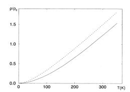
FIG. 3. Resistivity due to spin fluctuations as a function of temperature for the spin-fluctuation parameters  $T^*=110~{\rm K},$   $\alpha=0.55,\,\omega_D=1760~{\rm K},$  the electron parameters  $t=0.25~{\rm eV},$   $t'=0.45t,\,n=0.75,$  and the coupling constant  $g=0.64~{\rm eV}.$  Solid line: calculation with the improved ansatz Eq. (2.11). Dashed line: calculation with the standard ansatz Eq. (2.10).
