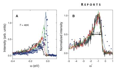
Fig. 3. (A) EDCs obtained in the  $(0,0) \to (\pi,\pi)$  direction after background subtraction. (B) EDCs scaled to the same peak position, showing that the overall shape scales linearly with binding energy. The peak width is approximately 1.5 times the binding energy in all spectra (double-headed arrow).
