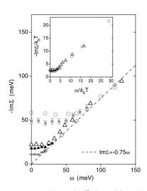
Fig. 4. A compilation of  $Im\Sigma$  obtained from  $\Delta k$  cuts or MDCs (solid symbols) and from peak widths in EDCs (open symbols) as a function of binding energy for 48 temperatures of K (diamonds), 90 K (triangles), and 300 K (circles). The inset shows the same data plotted in dimensionless units confirming scaling behavior. Error bars indicate uncertainties from the fits of MDCs to Lorentzian line shapes.
